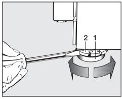
Once level, hold the foot 1 immobile using a wrench while turning the locking ring 2 to the right using a screwdriver. Turn each locking ring until it is tight against the bottom of the machine frame.
